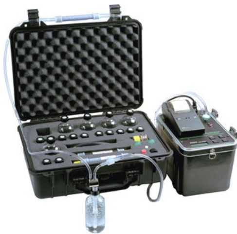
Fig. (2): Rad-7 H2O assembly with a 250 ml water sample
